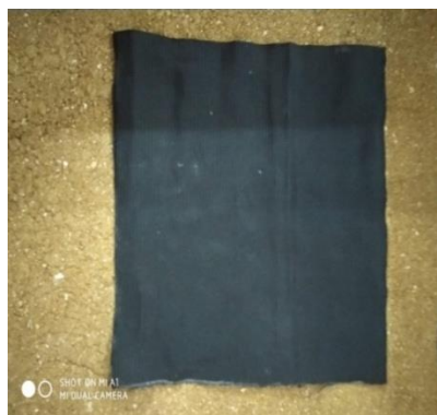
Figure .2 woven geotextile reinforcement
